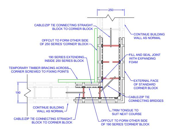
NOTE: ALTERNATE LH AND RH CORNER BLOCKS AS THE IS STACKED UP
