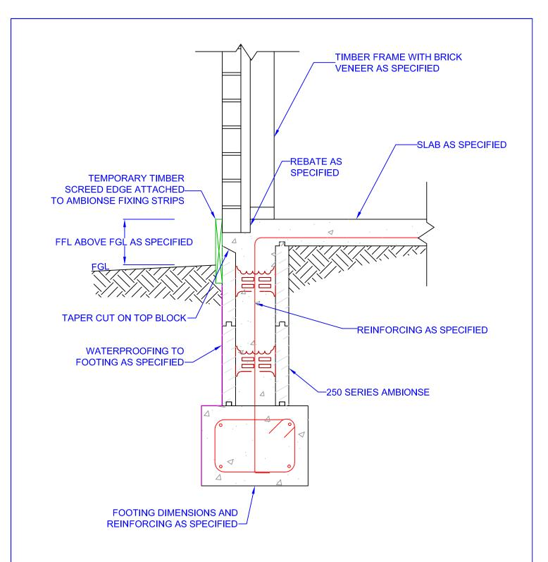
NOTE: TEMPORARY BRACING MAY BE REQUIRED ON FOOTING WALL TO ENSURE CORRECT ALIGNMENT
