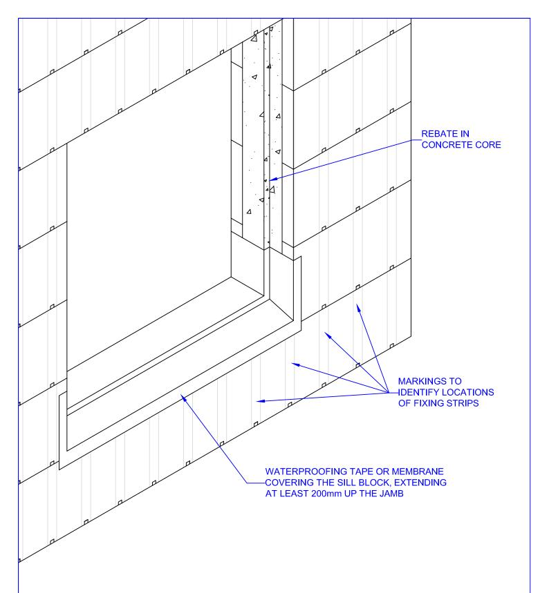
Note: THIS SHOWS THE OPENING READY TO RECEIVE THE JOINERY FOLLOWING THE CONCRETE POUR. REFER TO DRAWING CWD-HJ FOR INSTRUCTIONS ON FORMING THE REBATE
